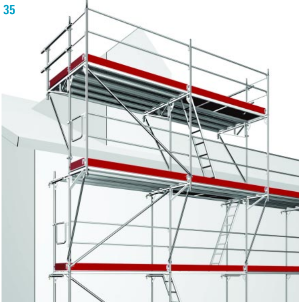
35 The assembly frames on the brackets must be secured with locking pins.
