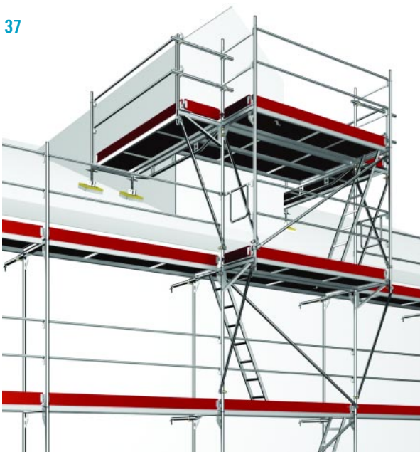
37 The side walls of dormers are easily scaffolded using SpeedyScaf aluminium U-double transoms. Assembly frames from the last scaffolding level must be secured with locking pins.
