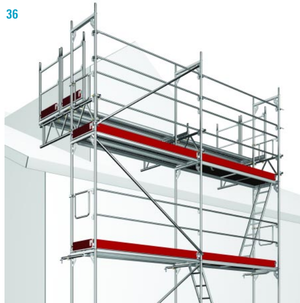
36 Connect lattice girders to the assembly frame and then fasten U transoms (with spigot and half-coupler Art. No. 1766.719) to it. Secure the assembly frames of the last and last-but-one levels using locking pins.
