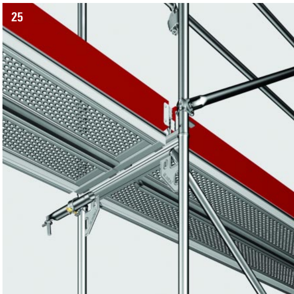
25 Anchoring with short wall tie
