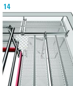
14 Version with 0.73 m bracket on the outside: If the scaffolding is widened with a 0.73 m bracket in the closing level, a flat and gap-free transition in the corner area is possible in conjunction with a 1.57 m long bay fitted at the end.
