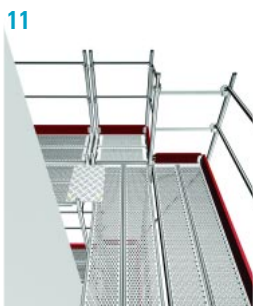
11 Widening at the top level is possible with the use of a swivelling and a fixed bracket together on one upright tube. This avoids any height mismatch in the scaffolding deck levels.
